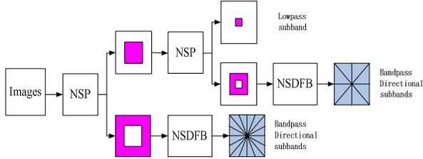
Figure 1. The structure of the NSCT
