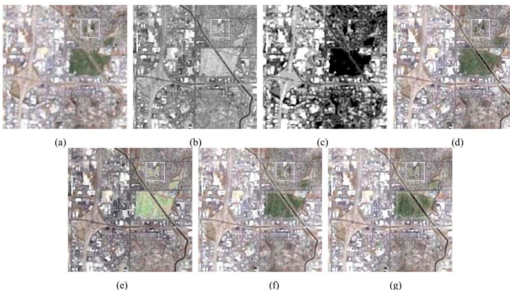
Figure 5. Source images and fused results with different methods: (a) the multi-spectral image. (b) the panchromatic image. (c) the region map of the intensity component of the multi-spectral image. (d) fused image by our method. (e) fused image by IHS transform method. (f) fused image by RWT method. (g) fused image by NSCT Simple method.
